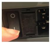
Power on the system using the switch on the back.
