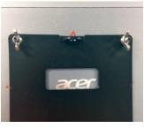
Remove the wing nuts from the back of the tablet.
