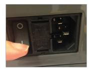
Power on the Labnet Enduro GDS II system using the switch in the back. Wait about 20 seconds before proceeding to the next step.
