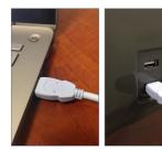
Connect the A-to-A USB cable to both the system USB and the computer. On the Labnet system, ensure the USB is plugged into the lower USB on the right hand side of the instrument.
