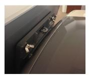
Secure the tablet in place with the wing nuts.
